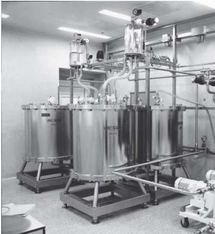
RFC installation processing 20,000 liters of human plasma every shift. Courtesy: Baxter
